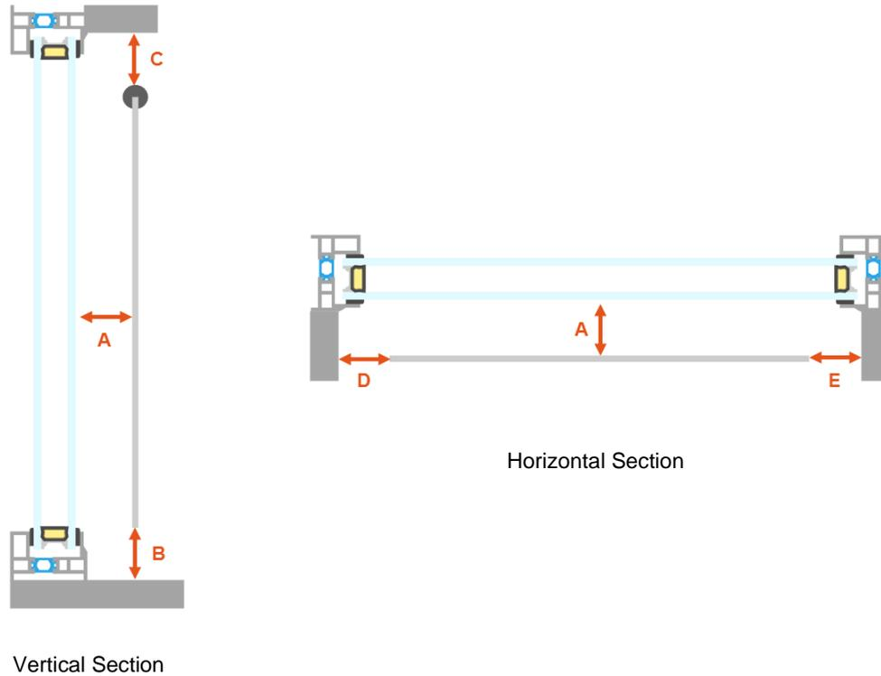
Figure 3 - Blind Ventilation Dimensions
