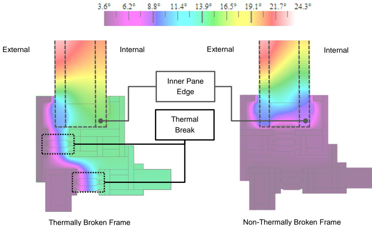
Figure 3 - Thermal Conductivity Through a Framing System
