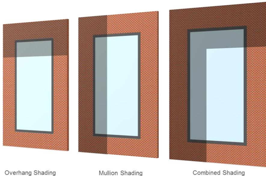
Figure 1 – Simple External Shading Patterns
