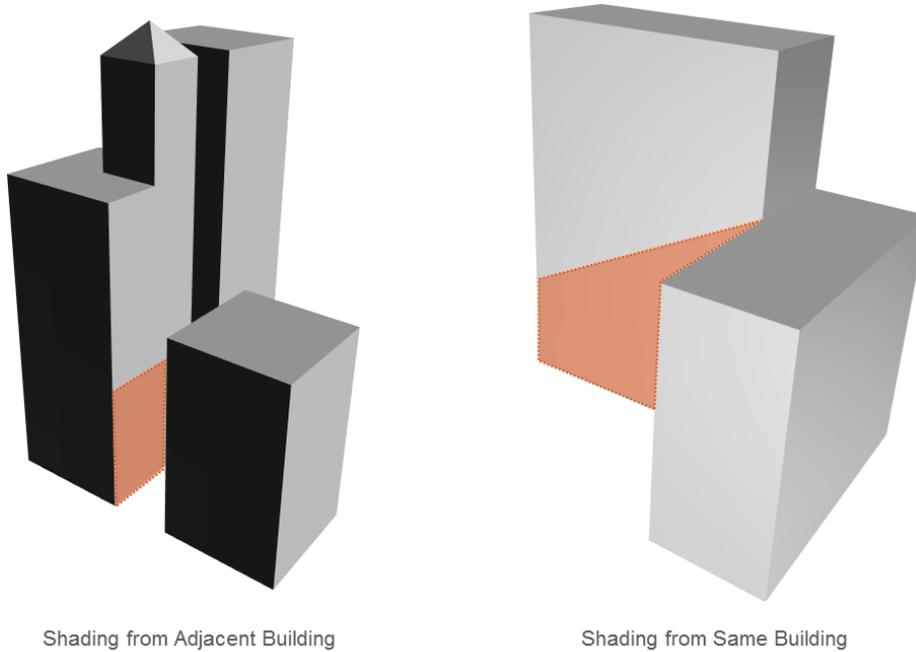
Figure 4 - Shading from Adjacent Structures
