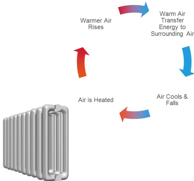
Figure 2 - Illustration of Thermal Convection
