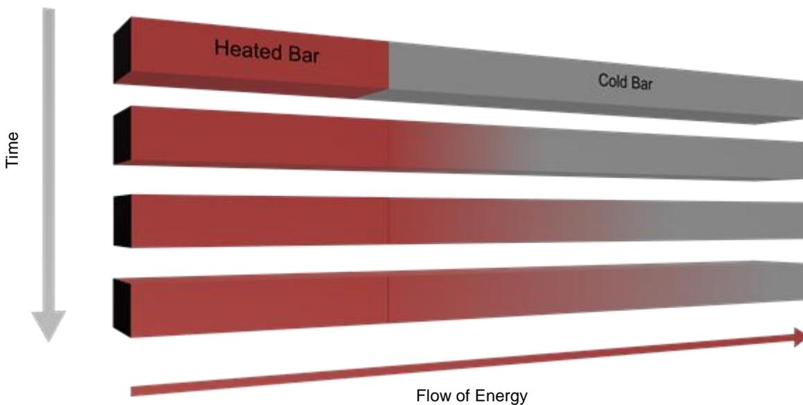
Figure 1 - Illustration of Thermal Conduction
