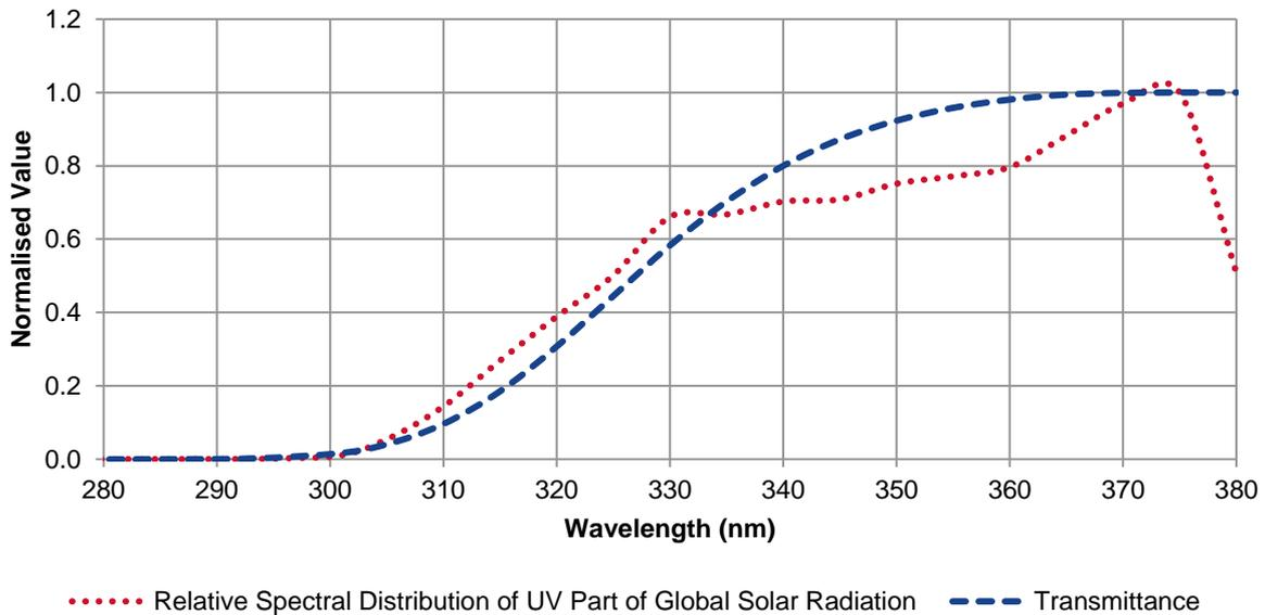
Figure 6 - Spectrally relevant parameters for the determination of UV transmittance
