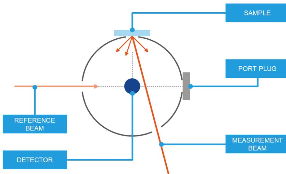
Figure 3 - Integrating Sphere Schematic (Reflectance)
