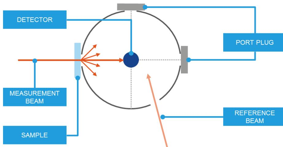
Figure 2 - Integrating Sphere Schematic (Transmittance)
