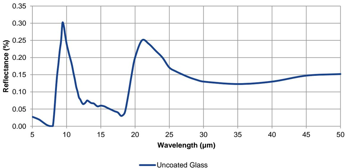
Figure 7 – Mid-IR, Far-IR Spectrum for Uncoated Glass
