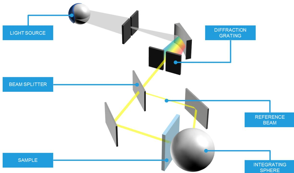
Figure 1 - Schematic of a Double-Beam Spectrophotometer with an Integrating Sphere
