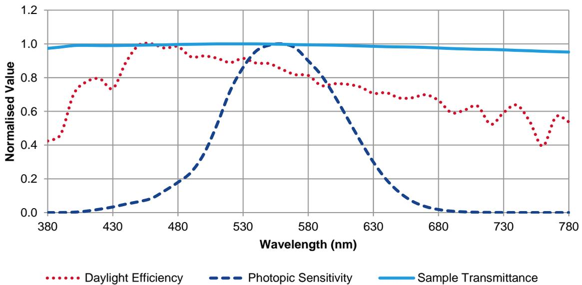
**Figure 4 - Spectrally relevant parameters for the determination of light transmittance**
