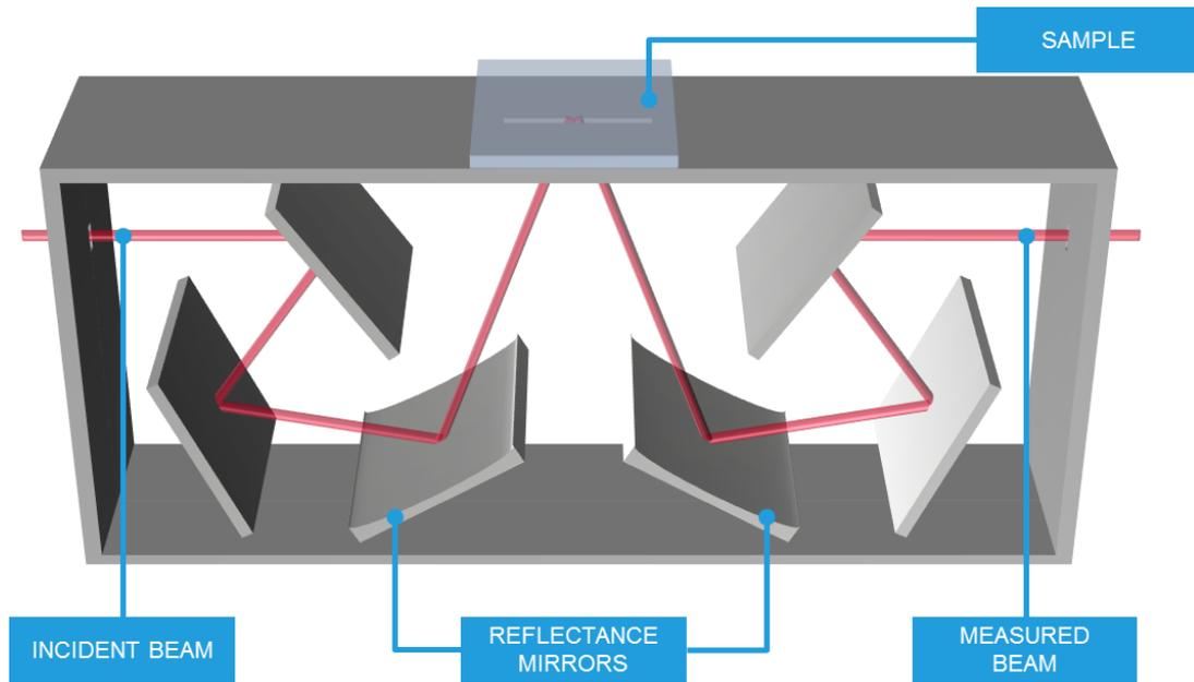
Figure 8 – Example of an IR Reflectance Setup
