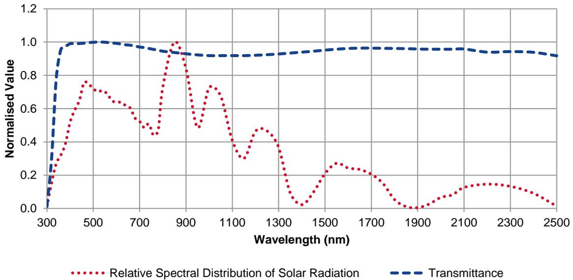
Figure 5 - Spectrally relevant parameters for the determination of energy transmittance
