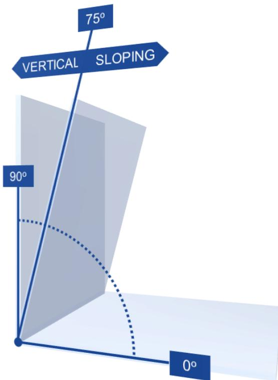
Figure 1 - Vertical/Sloping Glazing (Illustrative)
