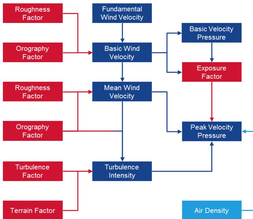
Figure 1 - Overview of Wind Load Determination
