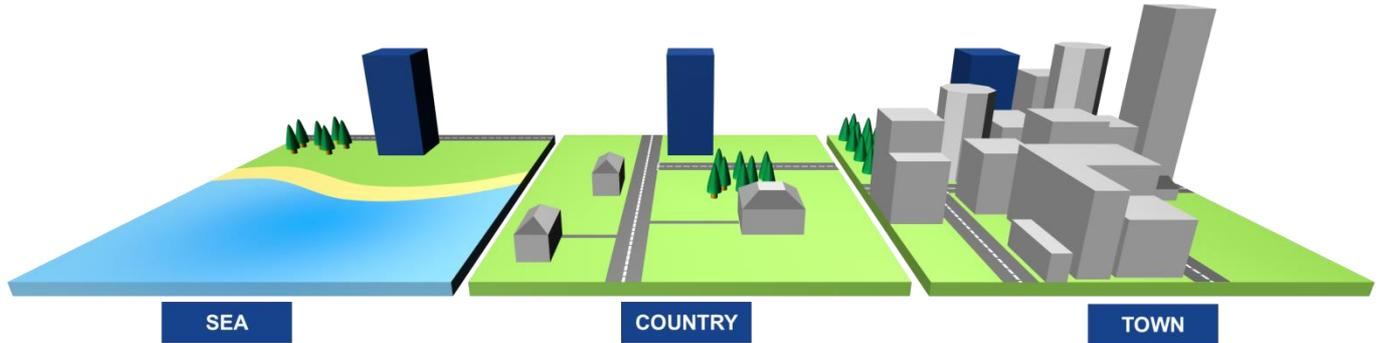
Figure 4 - Illustration of Terrain Categories
