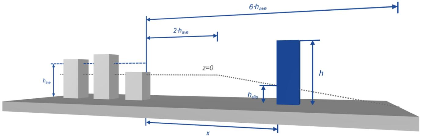
Figure 8 - Illustration for Upwind Building Distance
