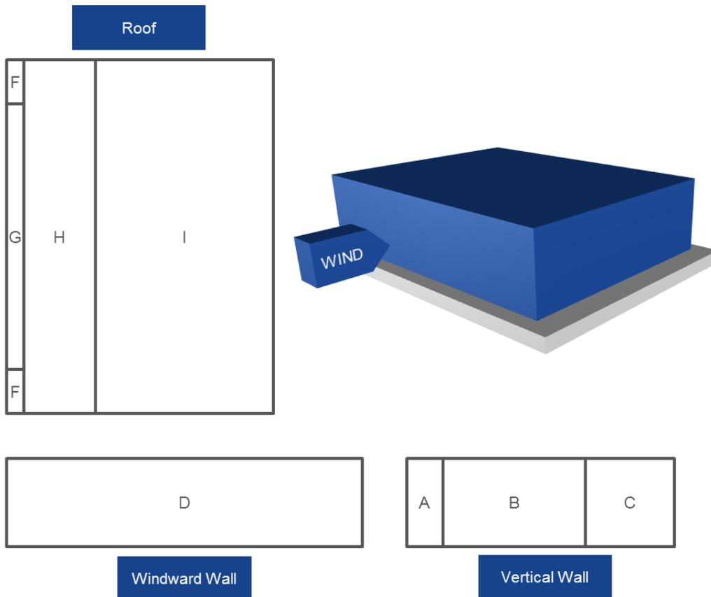
Figure 10 - Building Wall and Roof Zones
