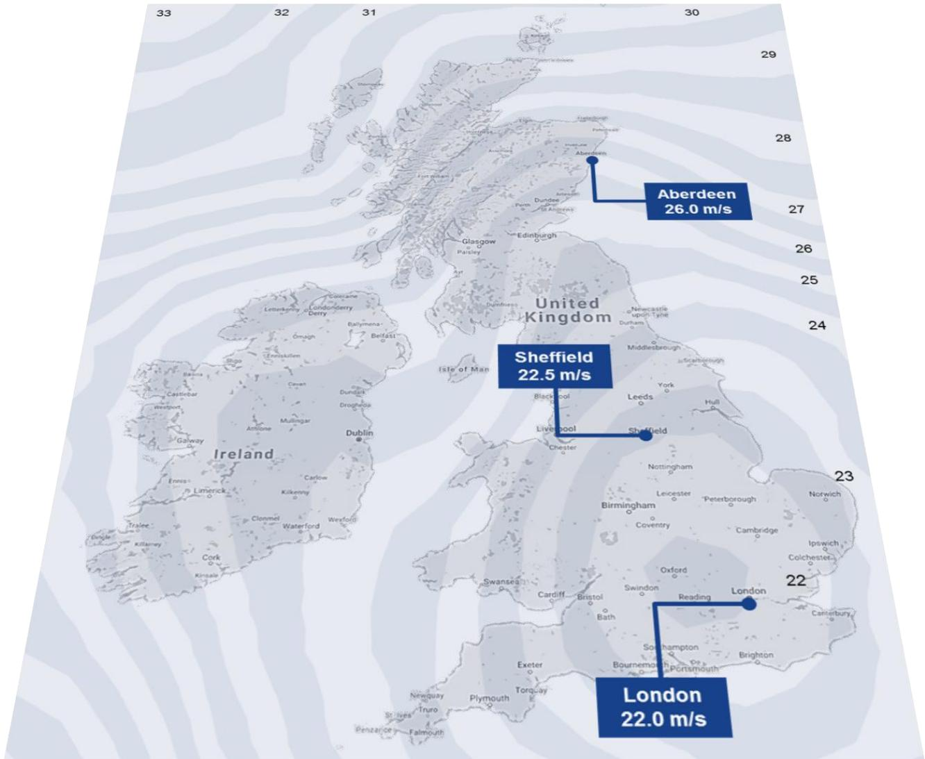
Figure 2 - Basic Wind Speed Zones
