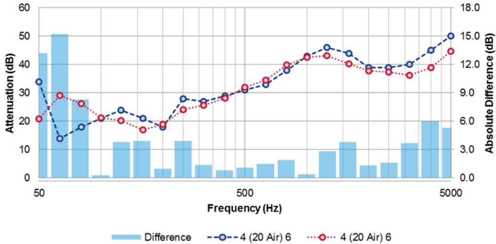
Figure 4 - 1/3 Octave centre band performance data, 4 (20 Air) 6
