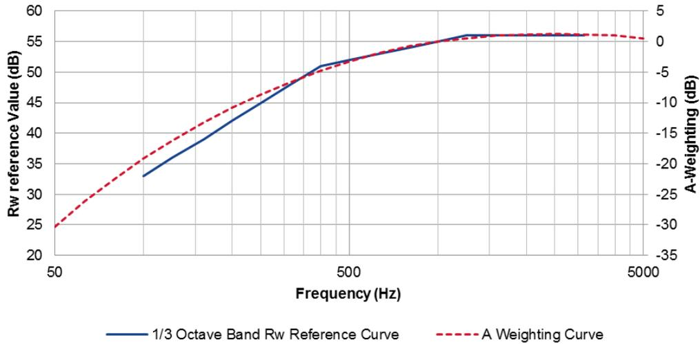
Figure 2 - Overlay of  $R_w$  reference curve & A-Weighting curve
